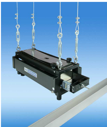
APS 113 with APS 8610 - Connecting Rod and APS 8611 - Steel Cable Kit prepared for Free Body Mode operation
