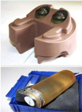
The **APTS sensors**, developed by IFSTTAR (French Institute of Science and Technology for Transport, Development and Networks) **for the "Q-Series" dummies**, are an essential new tool for the in-depth assessment of child restraint systems.
